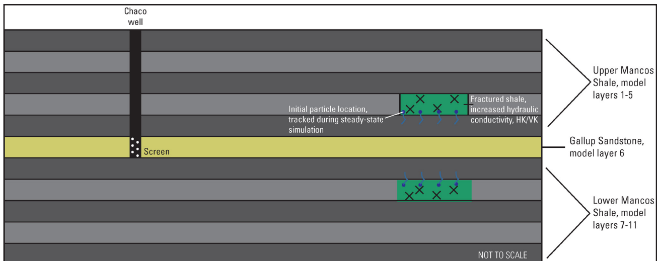
Figure 3. Conceptual depiction of hydraulic conductivity changes in hydraulic fracturing simulations within model layers.
